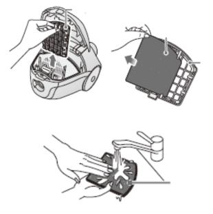
\*Make sure to dry filter before inserting
